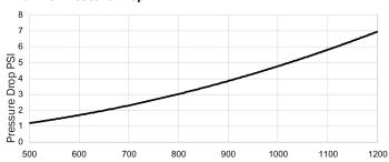
Flow in US GPM - SAE 10 @100°F Recommended pressure drop is 2 to 7 psi
